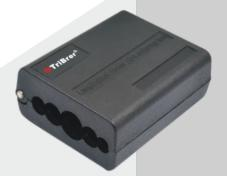
Stanlay TK-26 is a big mid span slitter with five grooves to sheath fiber optics from range of 4.5mm to 11mm. Fiber is places in the groove and the Cable Slitter is moved along the length to cut the sheath in two. cutting/slitting, provides 5 slots for dia 4.5mm, 6mm, 7mm, 8mm and 11mm.
